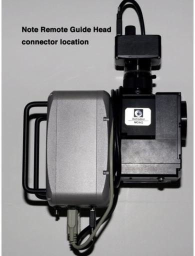
When using an SBIG STL-series camera with the SBIG remote guide head and an off-axis guider such as the Astrodon MOAG-A, be sure to orient the remote guide head so that its connector is closest to the STL body, as shown at left. Select "Off-axis Guided" for the guide method.
