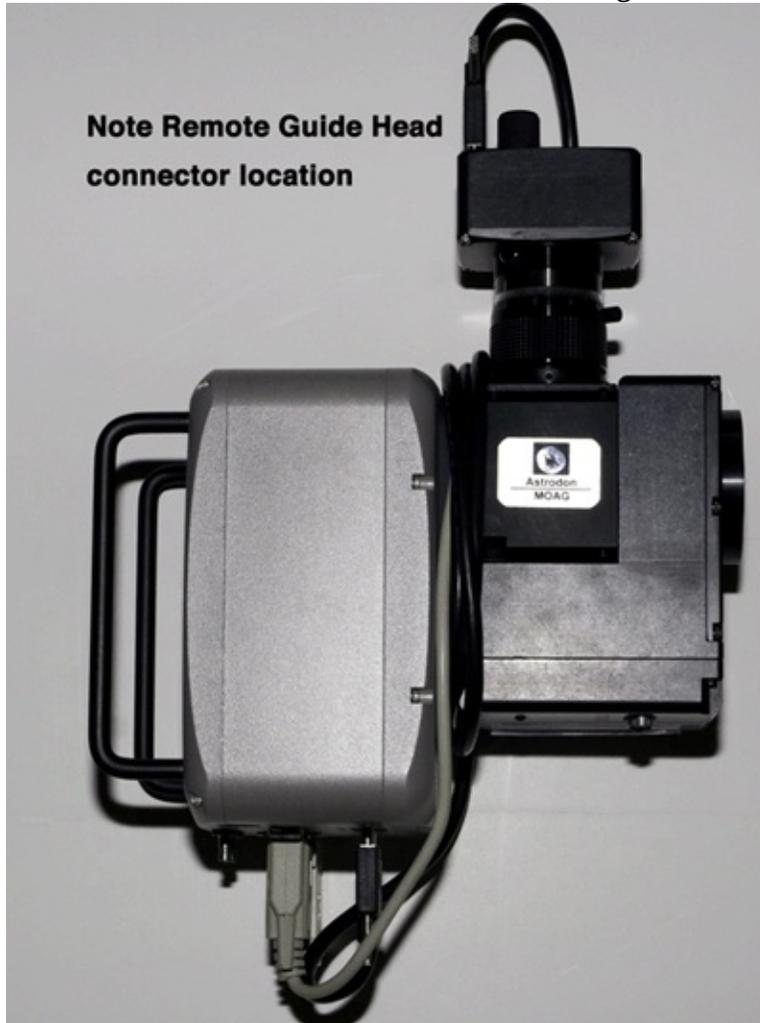
When using an SBIG STL-series camera with the SBIG remote guide head and an off-axis guider such as the Astrodon MOAG-A, be sure to orient the remote guide head so that its connector is closest to the STL body, as shown at left. Select "Off-axis Guided" for the guide method.
